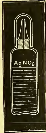
Test bottle, with capillary orifice. § 138.
